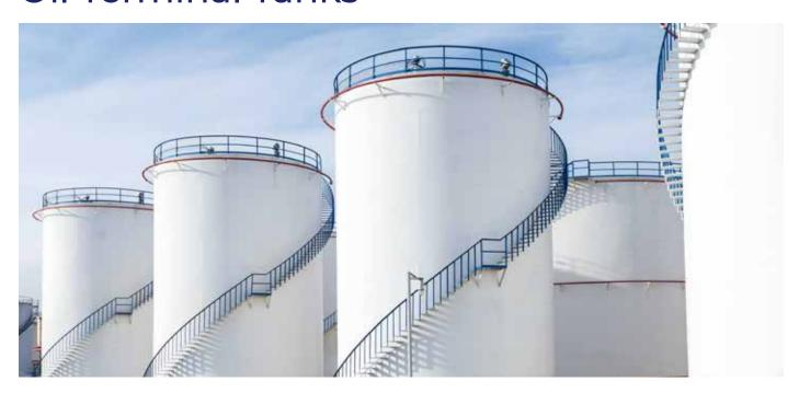
Storage tanks are commonly employed in oil and gas industry for the storage of fluids at different stages of the process and a variety of other industries consuming or producing liquids and vapors.
